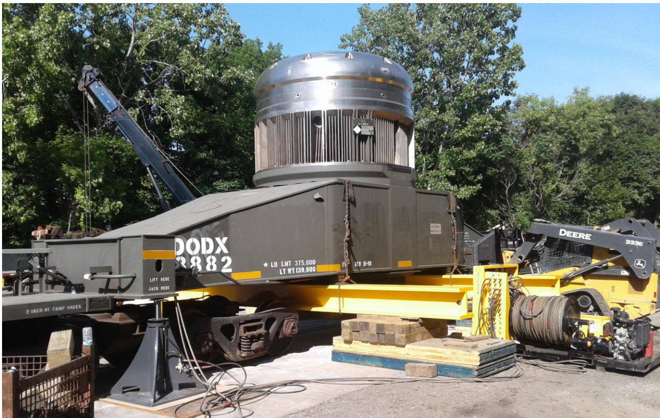
Figure 4: Shipping Container at the Ballston Spa Industrial Track Being Transferred from the Heavy Haul Vehicle
