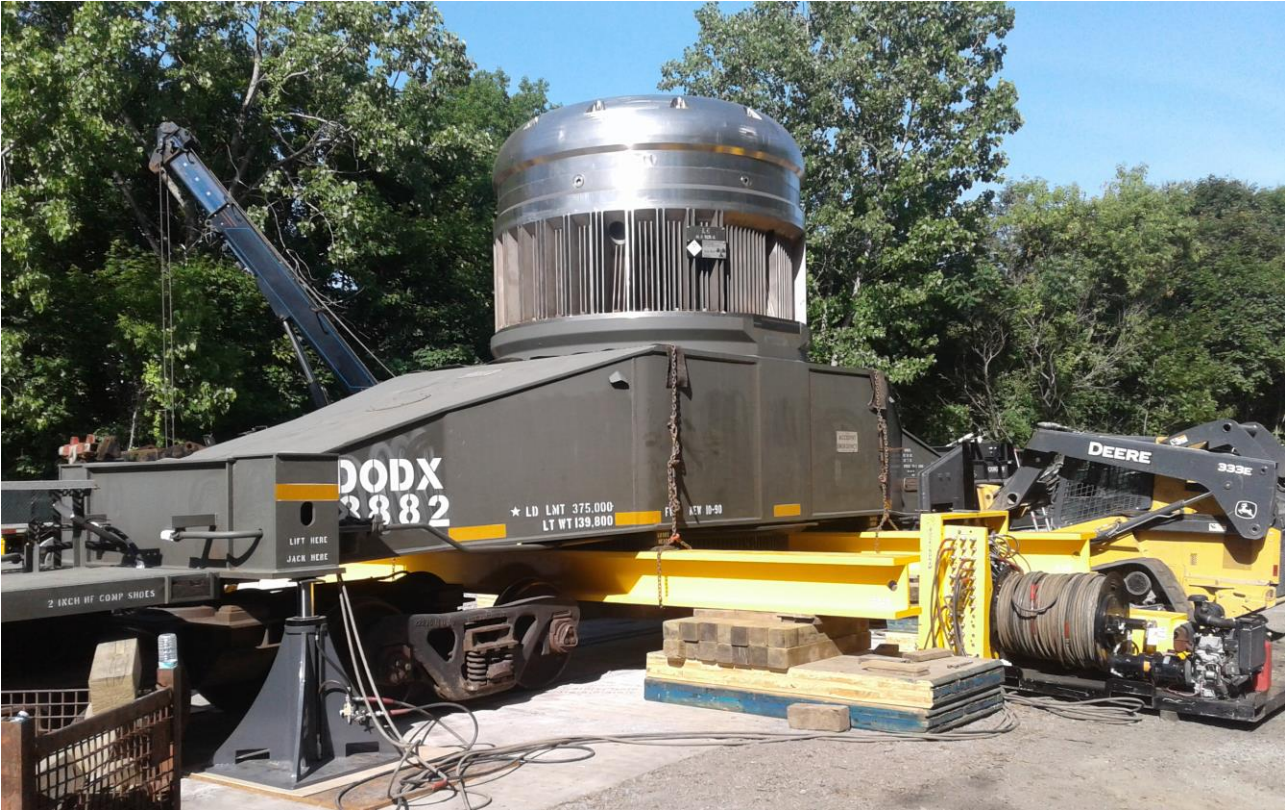
Figure 5: Shipping Container at the Ballston Spa Industrial Track Being Transferred to the Heavy Haul Vehicle
