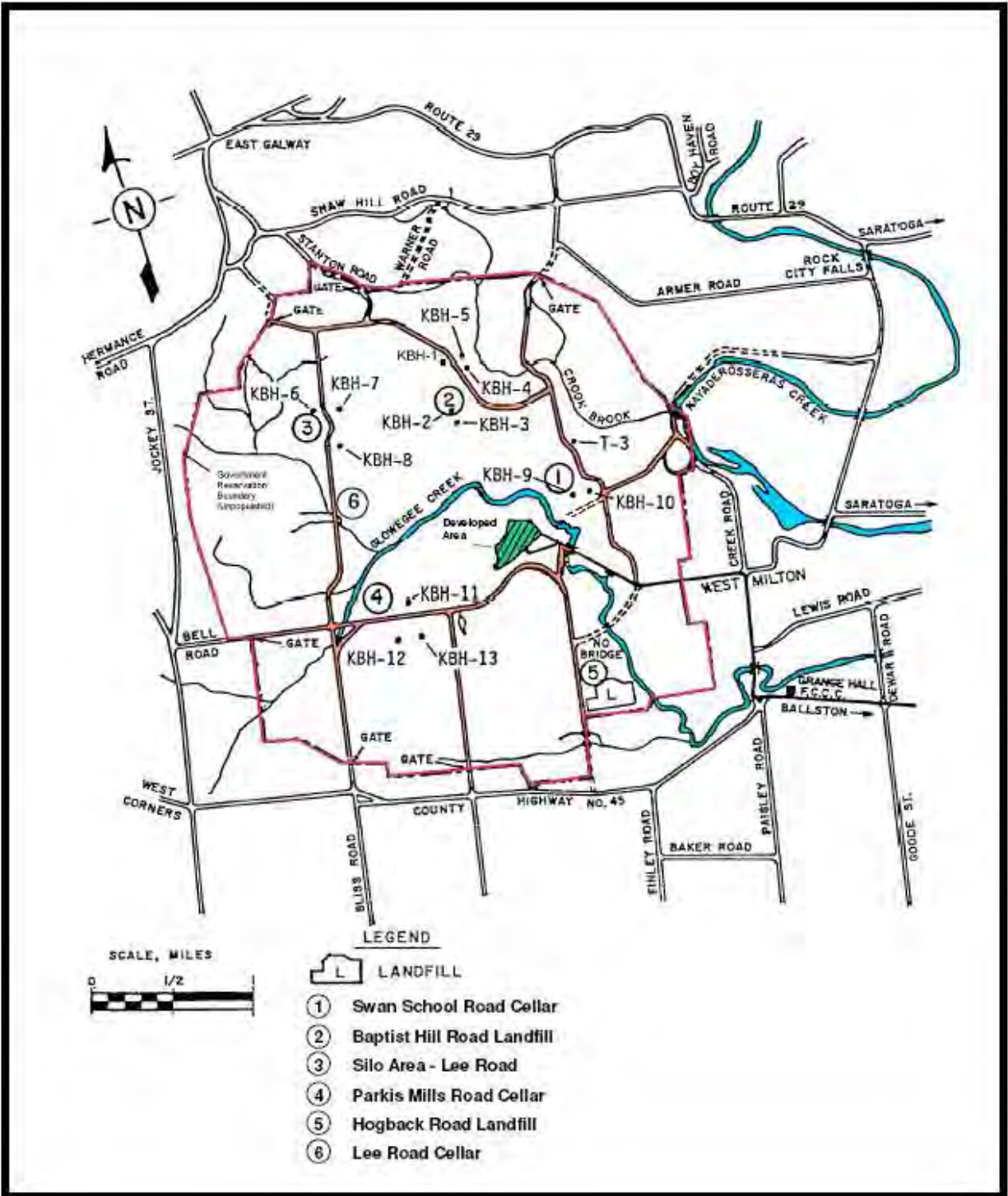
FIGURE 9 KESSELRING SITE, NEAR WEST MILTON, NEW YORK DISPOSAL AREAS – GROUNDWATER MONITORING WELLS
