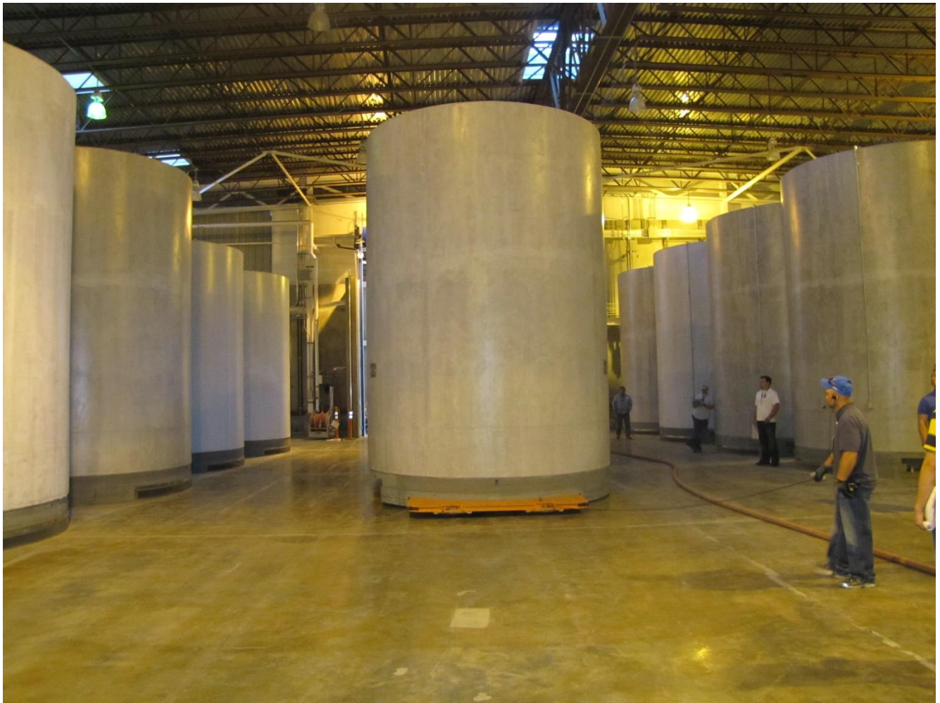
Figure 1. NRF workers move spent fuel in shielded concrete overpacks into storage.
